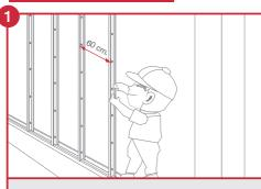
Fix studs to structural element no more than 60 cm. apart.
